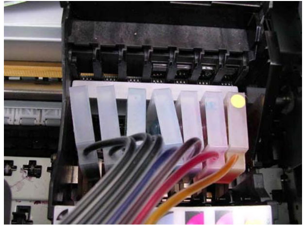
Fig. 15 Picture shows injectors fully installed in a 2100
